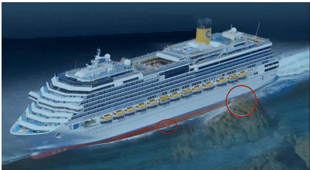
Figure 3 - Overview of the impact of the Costa Concordia with the Scole rocks. The points where the ship collides with the rocks are highlighted by red circles (Source: Judgment of the Court of First Instance of 11 February 2015 no. 115/2015).
